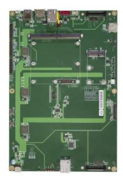
**ESMC-CTI01-EVM SMARC Carrier Board:** Also available is the ESMC-CTI01-EVM Carrier Board. It is generally used for evaluation and development when using the SMARC module by breaking out specific connectors and capabilities to facilitate testing and development.
